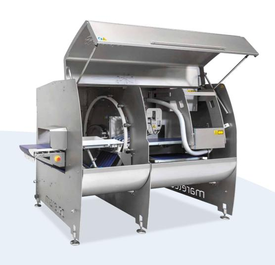
A PORTIO 3 adds two lateral cameras to the PORTIO 1. This allows the machine to improve the scanning and cover blind spots at the side of the product that cannot be detected by the top camera only. It is used for accurate portioning red meat, whole fish or any product with an irregular shape, in a vertical way. The machine can be equipped with the options mentioned on page 20.
