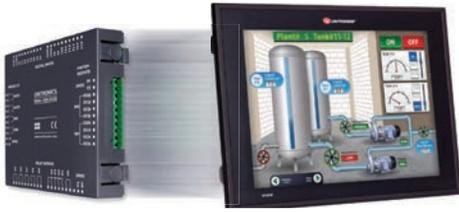
Plug a Snap-in module directly into the back of a Vision PLC.
