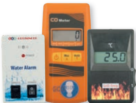
Examples of printed housings
