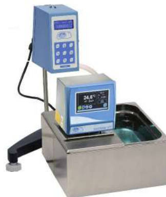
Immersion thermostat Digiterm controlling temperature of viscometer.
